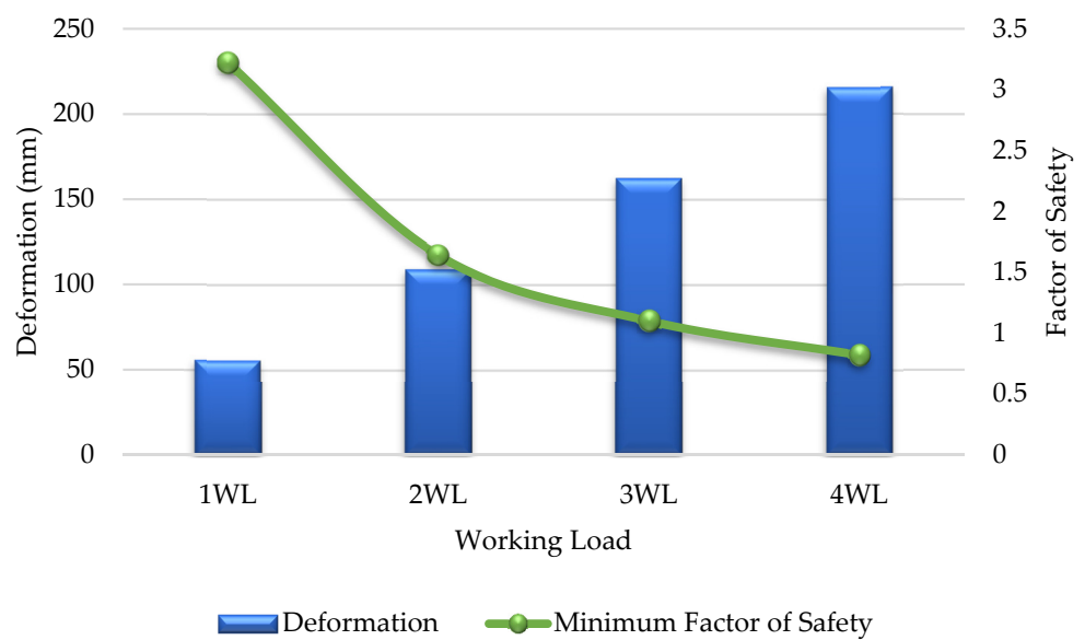
Figure 10. Deformation and Factor of Safety (FOS) for GFRP cross-arm (broken wire condition).
