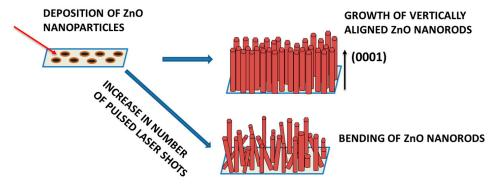
**Figure 8.** Schematic diagram of growth of vertically aligned ZnO nanorods (VAZO) by using high pressure assisted pulse laser deposition (PLD) process.
