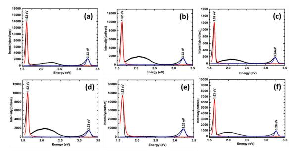
**Figure 5.** PL spectra of ZnO nanorods grown by using 5000 pulsed laser shots at different temperatures (a) 500 °C, (b) 550 °C, (c) 600 °C and PL spectra of ZnO nanorods grown at 550 °C by varying the number of pulse laser shots (d) 5000, (e) 10,000, (f) 15,000.
