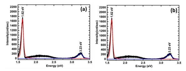
**Figure 6.** PL spectra of ZnO nanorods grown at 500 °C and annealed in (a) O<sub>2</sub> atmosphere (b) H<sub>2</sub> atmosphere.
