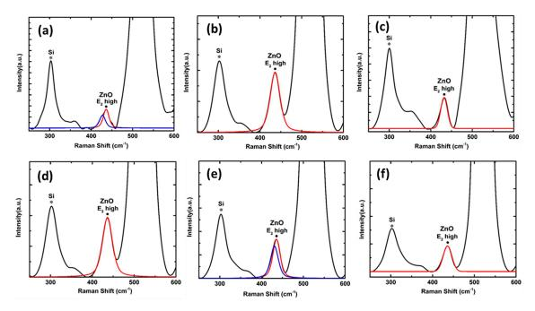
**Figure 3.** Raman spectra of ZnO nanorods at different temperatures (**a**) 500 °C, (**b**) 550 °C, (**c**) 600 °C and Raman spectra of ZnO nanorods grown at 550 °C by varying the number of pulsed laser shots (**d**) 5000, (**e**) 10,000, (**f**) 15,000.
