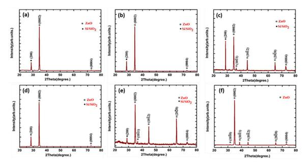
**Figure 2.** XRD spectrum of VAZO nanorods grown on Si substrate at **(a)** 500 °C, **(b)** 550 °C, **(c)** 600 °C and XRD spectrum of VAZO nanorods grown on Si substrate at 550 °C by varying the number of shots **(d)** 5000, **(e)** 10,000, **(f)** 15,000.
