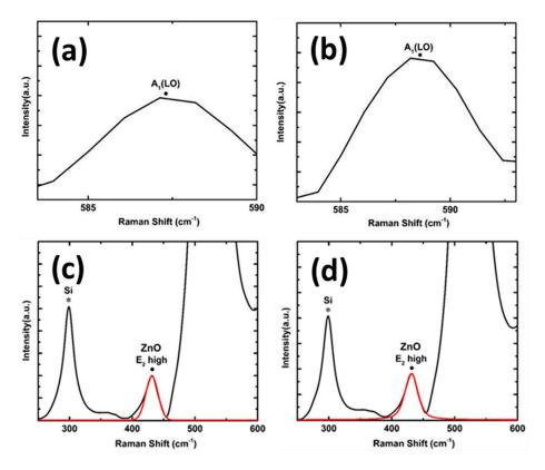
**Figure 4.** A<sub>1</sub> (LO) mode in Raman spectra of aligned ZnO nanorods at (a)  $500 \,^{\circ}$ C (b)  $550 \,^{\circ}$ C and E<sub>2</sub> high mode of aligned ZnO nanorods grown at  $500 \,^{\circ}$ C, annealed in (c) O<sub>2</sub> atmosphere (d) H<sub>2</sub> atmosphere.
