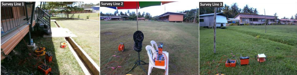
Photo 1. Terrameter SAS4000 in progress acquiring data from LPS area.
