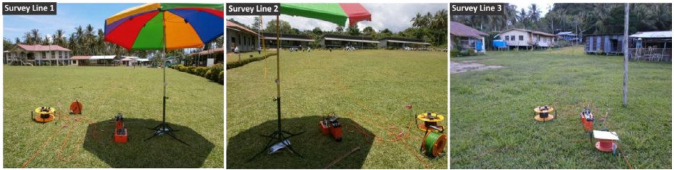
Photo 2. Terrameter SAS4000 in progress acquiring data from PPS area.
