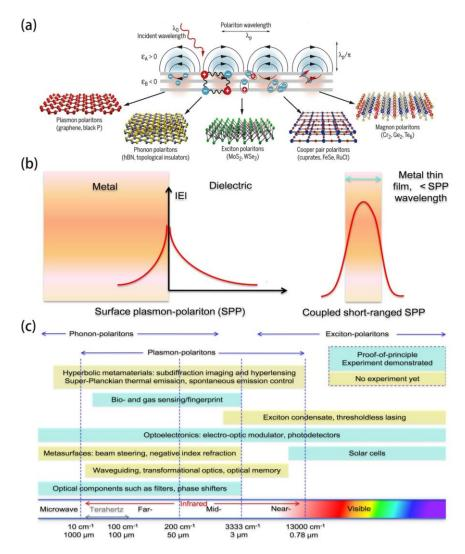
**Figure 1.** (**a**) Schematic of the formation of polaritons in various vdW materials. (**b**) Schematic explanation of surface plasmon-polaritons in metal and 2D materials. (**c**) Summary of potential applications of polaritons (plasmons, phonons, excitons) in 2D materials and their working frequency ranges. (**a**) Reproduced with permission [43], Copyright 2016, AAAS.
