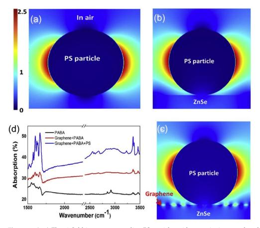
**Figure 3.** (**a**–**c**) Electricifield images surrounding PS particles with an excitation wavelength of 5460 nm, for PS particle in air (**a**), on a ZnSe substrate (**b**), and on graphene/ZnSe (**c**), respectively. (**d**) Mid-IR absorption spectrum for a higher density of PABA on ZnSe (black), graphene/ZnSe (red) and graphene/ZnSe/PS (blue). (**a**–**d**) Reproduced with permission [71], Copyright 2017, Pergamon-Elsevier Science Ltd.
