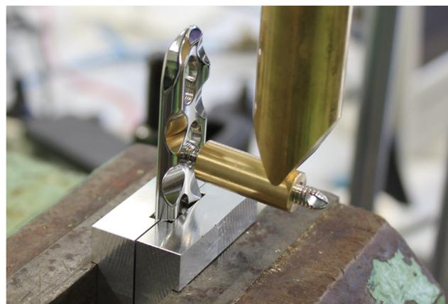
Fig. 3. Test setup for the locking compression construct.
