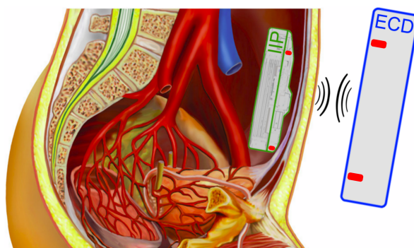
Figure 10. Schematic representation of the inductive link application, with the External Controlling Device (ECD) outside the body (blue), the Implantable Infusion Pump (IIP) inside the abdominal cavity (green) and the indicated transmission coils (red).
