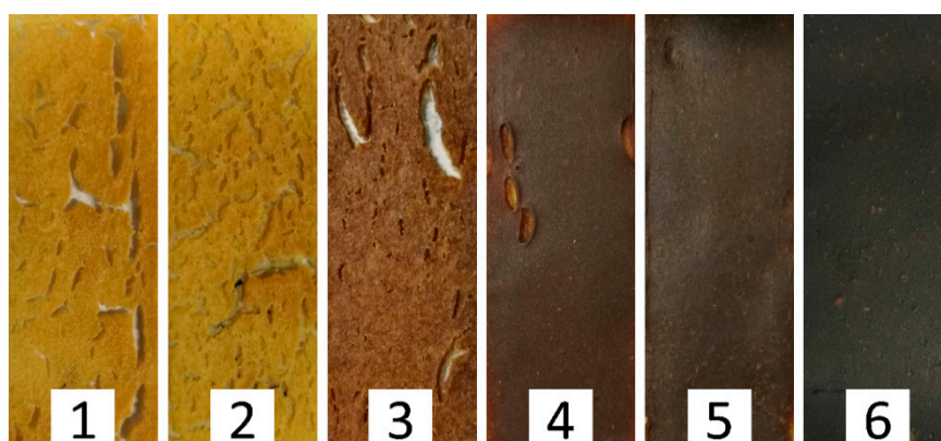
Figure 4. The toughness evaluation of the different adhesives 1: SM, 2: SM/TGIC, 3: SM/TGIC/DAS-5, 4: SM/TGIC/HD-2.5, 5: SM/TGIC/HD-5, and 6: SM/TGIC/HD-7.5.
