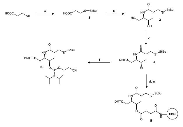
*Reagents and conditions*: (a) Di-*tert*-butyl-1-(*tert*-buthylthio)-1,2-hydrazinecarboxylate, triethylamine, DMF; (b) L-threoninol, EDCI, 1-hydroxybenzotriazole, diisopropylethylamine, DMF; (c) dimethoxytrityl chloride, pyridine; (d) succinic anhydride, N,N-dimethylaminopyridine, pyridine; (e) long chain amino alkyl-controlled pore glass (LCAA-CPG), TBTU, triethylamine, ACN; (f) 2-cyanoethyl-N,N-diisopropylaminochlorophosphine, diisopropylethylamine, CH<sub>2</sub>Cl<sub>2</sub>.
