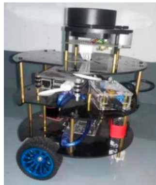
Figure 8. The designed mobile robot with 2D lidar.
