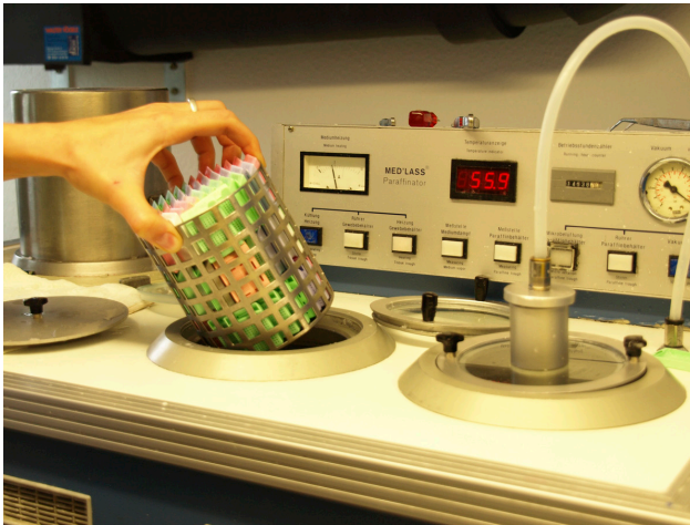
Figure 8. Following dissection of specimens, many tissue cassettes with biopsy specimens of different patients are put in a basket and are processed in a tissue processor in order to dehydrate them and to prepare them for paraffin embedding. [Copyright: ©2014 Weyers.]
