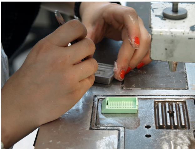
Figure 9. Following procession of tissue, tissue cassettes are taken out of the tissue processor and are once again arranged in a row according to ascending pathology numbers. Paraffin blocks are arranged in the same fashion. The pathology numbers on tissue cassettes and blocks must be checked for concordance before opening the next cassette. Only one cassette should be opened at a time. Pincers must be cleared before taking out the next specimen in order to prevent transmission of fragments of tissue into a wrong block. [Copyright: ©2014 Weyers.]
