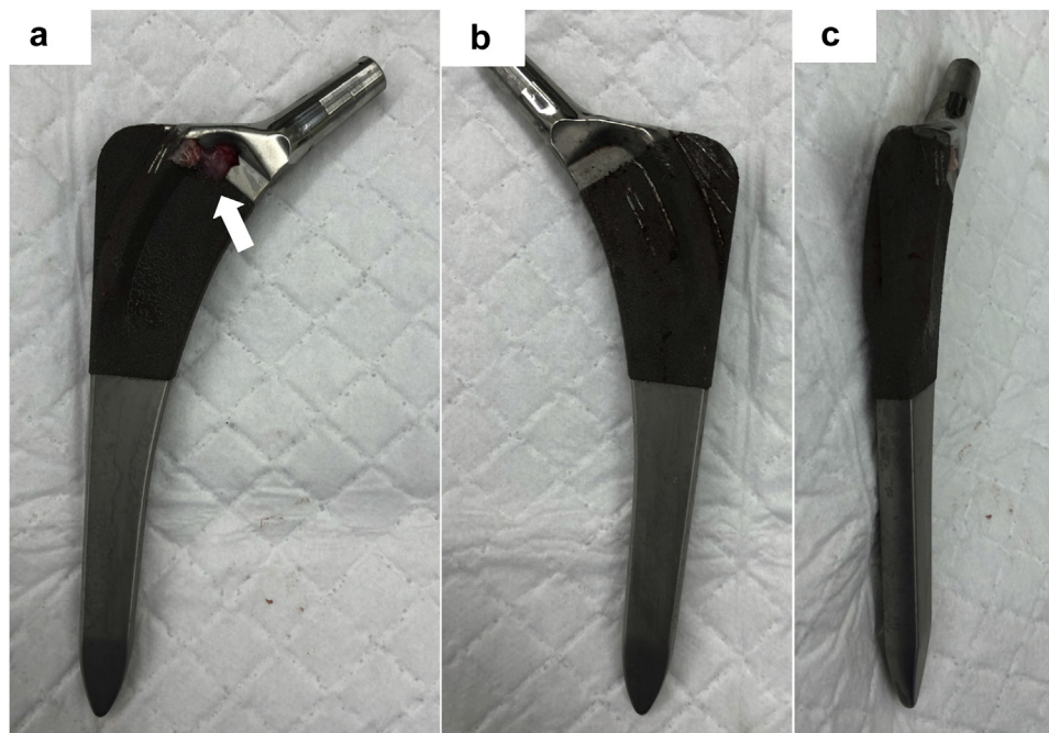
Figure 5. The removed implant showed very limited osseointegration at the proximal end of the stem (white arrow). (a) front, (b) back, and (c) lateral.
