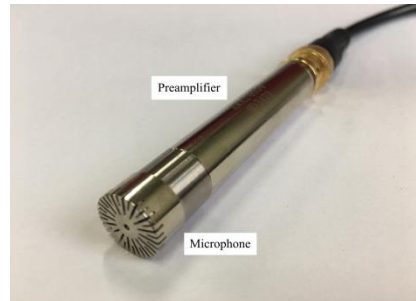
Figure 9. Structure of acoustic sensor.
