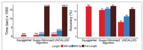
**Fig. 6** Processing time and accuracy comparison. The processing time of SquiggleNet with 300 bp of input is among the lowest, and yet the accuracy is the highest among the three methods. For the other two alignment-based methods, with longer input length, the processing time grows drastically, whereas the accuracy gain is limited
