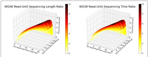
**Fig. 8** Throughput and sequencing time comparison without/with read-until. When the average non-target read length is about 20 times longer than the target read length, and sample contains over 90% non-target reads, a normal sequencing pipeline would have to sequence  $\sim$  10 times more base pairs (left) than Read-Until pipeline with SquiggleNet to achieve a fixed number of targeted reads. The ratio is about 10 for the required sequencing time as well (right)
