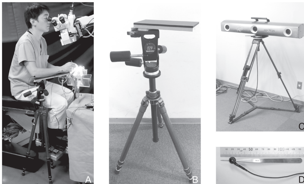
Fig. 1 A: Panoramic photograph of our experimental environment simulating microneurosurgery. Skull and cerebrum models were installed in a Sugita multipurpose head frame and head holder attached to an operating table. The neurosurgeon sits on an operator's chair and observes the cerebrum model through an operating microscope. His right forearm and the hypothenar eminence are placed on an armrest seated beside the operator's chair. B: Handmade experimental armrest. It was designed to support the subject's forearm and hand from the elbow to the hypothenar eminence. The armrest was mounted on a tripod. C: The camera unit of the three-dimensional optical coordinate measuring machine that was used in this study (K600; Nikon Metrology NV, Leuven, Belgium). D: A dedicated infrared light-emitting diode marker of the coordinate measuring system pasted on a pair of surgical forceps.
