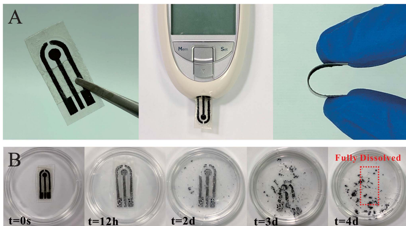
Fig. 2 (A) Images of the fully transient electrochemical strips. (B) Sequential dissolution images of a fully transient electrochemical strip in DI water (RT).
