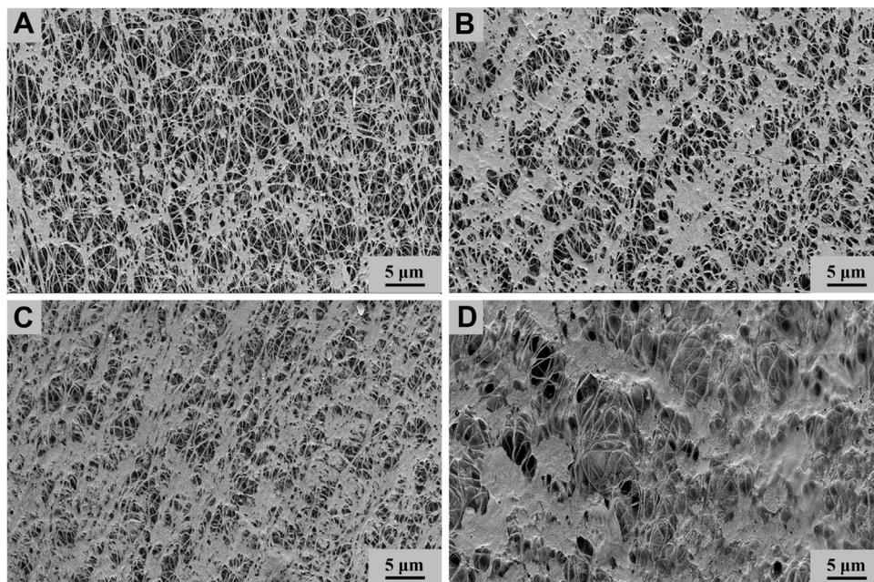
**Fig 3.** Scanning electron microscope images of the surface of the endograft without coating (A) and with the coating containing 0.1  $\mu\text{g}/\text{mm}^2$  (B), 0.3  $\mu\text{g}/\text{mm}^2$  (C), and 3.6  $\mu\text{g}/\text{mm}^2$  (D) paclitaxel (original magnification  $\times 2000$ ).
