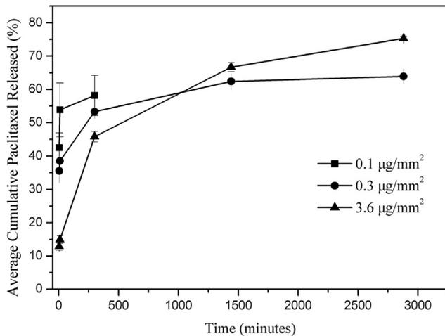
**Fig 4.** In vitro release curves (presented as the mean  $\pm$  standard deviation) for the endograft with poly(lactide) and paclitaxel coating containing  $0.1 \mu\text{g}/\text{mm}^2$  (squares),  $0.3 \mu\text{g}/\text{mm}^2$  (circles), and  $3.6 \mu\text{g}/\text{mm}^2$  (triangles) paclitaxel.
