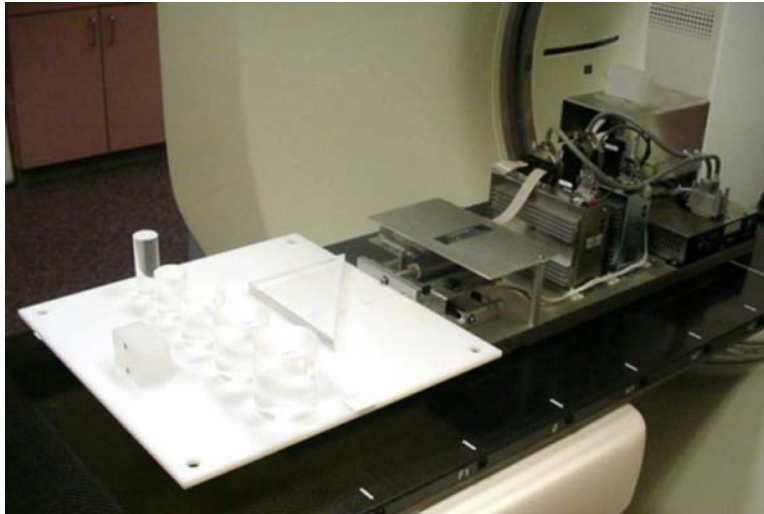
FIG. 2. The motion platform used in this study. Cylindrical phantoms were placed on the platform, together with the Varian Real-Time Position Management system marker block, and moved periodically along the longitudinal axis of the phantom (in and out the scanner bore).
