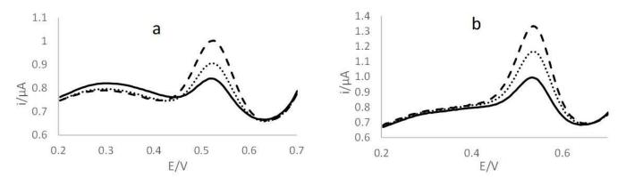
**Figure 2.** Voltammograms obtained using the portable kit for (a)  $Hg_{IN}$  and (b)  $CH_3Hg$  quantification: — tuna fish; ···· first addition (5  $\mu$ g  $L^{-1}$ ); - - - - second addition (10  $\mu$ g  $L^{-1}$ ).
