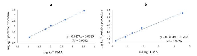
**Figure 3.** Correlation between the concentrations (mg kg<sup>-1</sup>) of (a) Hg<sub>TOT</sub> and (b) CH<sub>3</sub>Hg obtained using the portable procedure and DMA.  $\bullet$  = samples (tuna fish 2, tuna fish 1, blue marlin, swordfish 1 and swordfish 2, reported in ascending order of concentration).
