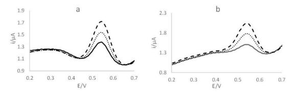
**Figure 1.** Voltammograms obtained using the portable kit for (a) Hg and (b) CH<sub>3</sub>Hg quantification: —, ERM-CE 464; …, first addition (5  $\mu$ g L<sup>-1</sup>); - - - -, second addition (10  $\mu$ g L<sup>-1</sup>).
