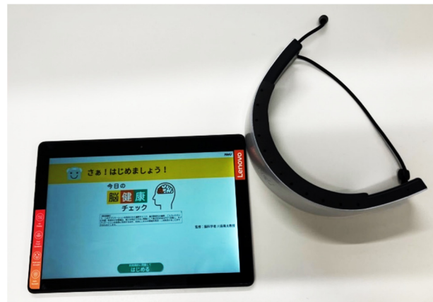
Figure 3. Measurement device. Figure 3 shows the HOT-2000 and the tablet that performed the TMT (for Japanese).
