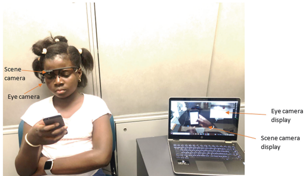
Fig. 1 The experimental set-up showing the wearable eye tracking headset (Pupil Labs GmbH Berlin, Germany) during smartphone use. The eye camera display of the participant's eye and the scene camera display enabling continuous monitoring of participant adherence by the examiner on the laptop. Child and parental consent were obtained for use of this image.
