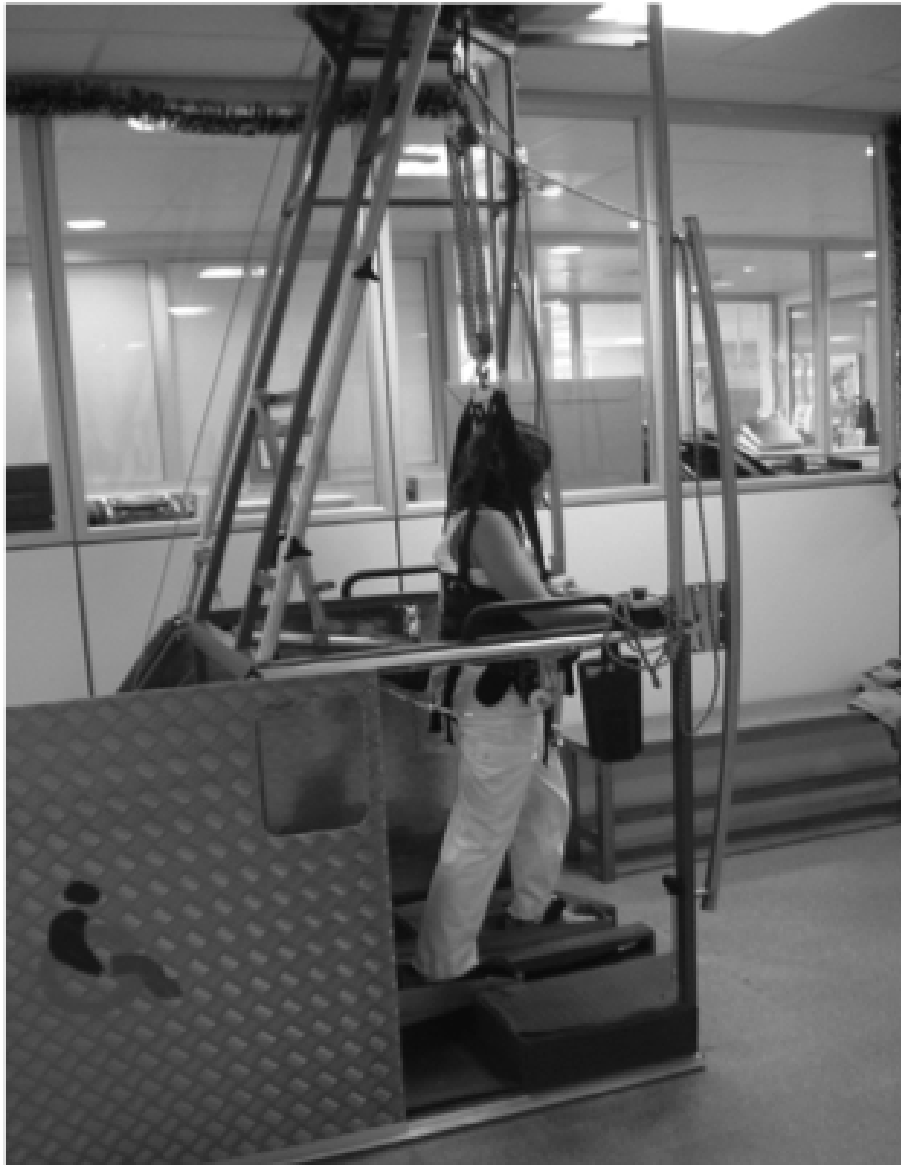
Figure 2 A sub-acute stroke patient during the Robotic Gait training session. During the Body-Weight-Supported-Robotic-Gait Training (BWSRGT) the body weight is slightly unloaded via the use of a harness, while the fixed foot placement on the device ensures a set pattern that mimics human gait with alternate stance and swing phase.
