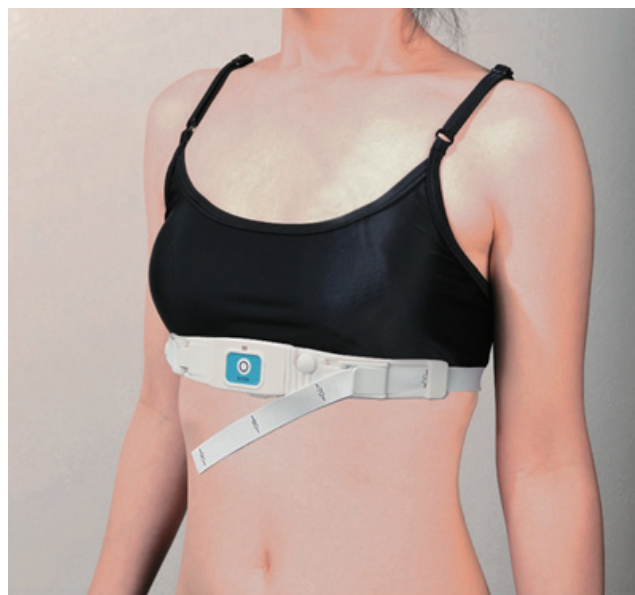
Fig. 1. The chest strap-style monitor for 7-day Holter ECG monitoring
