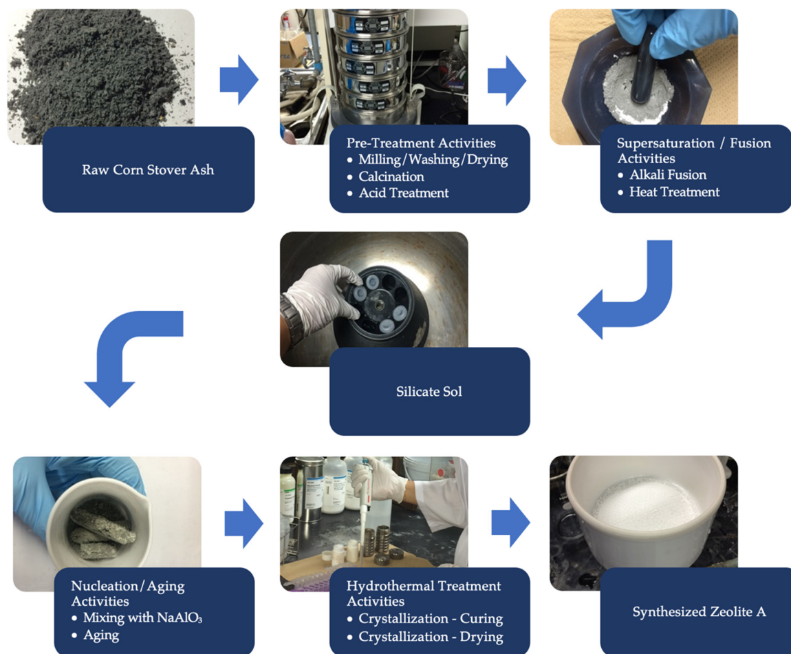
Figure 2. A schematic representation for the two-step zeolite A preparation method using corn stover ash.
