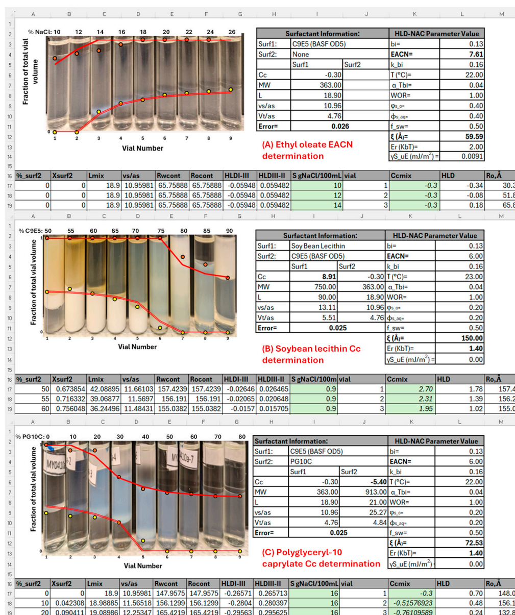
Figure 1. (A) Salinity scan used to obtain the Equivalent Alkane Carbon Number (EACN) of ethyl oleate (oil) using pentaethylene glycol nonyl ether (C9E5 or OD5, surfactant 1); the numbers on top of each vial represent the %w/v NaCl (salinity) in the aqueous phase. (B) Surfactant composition scan with lecithin (SBlec, surfactant 1) and reference surfactant C9E5 (surfactant 2) using limonene (EACN = 6) as oil and a 0.9% w/v NaCl aqueous phase; the numbers on top of each vial represent the wt% of C9E5 (surf2) in the mixture with lecithin (wt%surf1 = 100 – wt%surf2). (C) Surfactant composition scan with reference surfactant C9E5 (surfactant 1) and polyglycerol-10 caprylate (PG10C, surfactant 2) using limonene (EACN = 6) as oil and a 0.9% w/v NaCl in the aqueous phase; the numbers on top of each vial represent the wt% of PG10C (surf2) in the mixture with C9E5 (surf1). The orange and yellow dots are the experimental determination of the lower level (LL) and upper level (UL) boundaries of the \mu E phases. The solid red lines are predictions of the lower level (LL) and upper level (UL) boundaries of the \mu E phases predicted by the HLD–NAC programmed in the HLD–NAC tutorial [16], using the algorithm explained in Figure 2.
