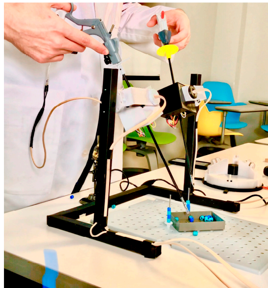
Figure 6. Developed system instrumented with force and motion-tracking sensors during the proposal validation with the use of common laparoscopic instruments.
