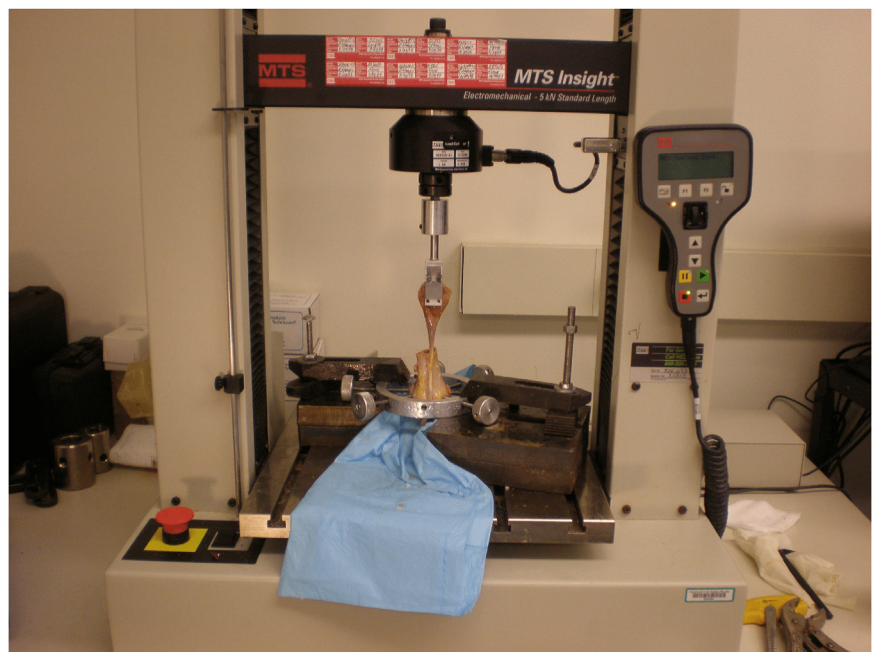
Fig 5. Materials testing system for tendon constructs.
