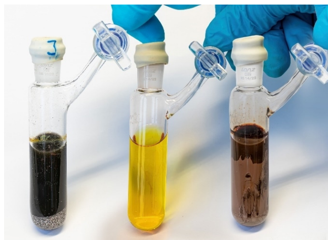
Figure 1. From left to right: (2-Ethylhexyl)sodium ( 1 ) in hexane prepared in batch over metallic sodium, 5 min after addition of 2 . (2-Ethylhexyl)sodium ( 1 ) in hexane prepared via a sodium-packed-bed reactor, 5 min after collecting. (2-Ethylhexyl)sodium ( 1 ) in hexane prepared via a packed-bed sodium reactor, 18 h after collecting.
