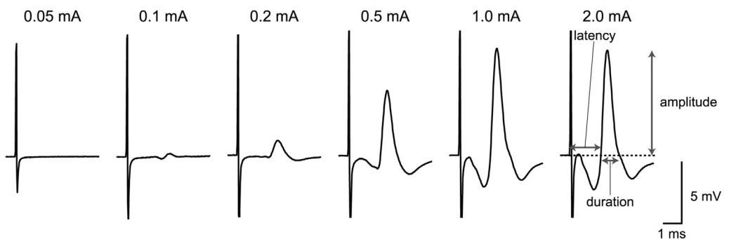
Fig. 4. Representative CMAP traces and measurable parameters.
