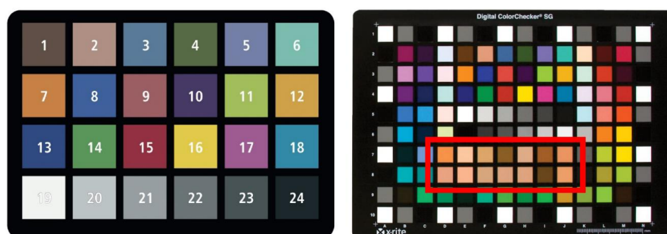
Figure 2. ColorChecker Classic (left, full-range CCT) and Digital SG (right, skin-range CCT). Skin patches used in our study are placed inside the red square.
