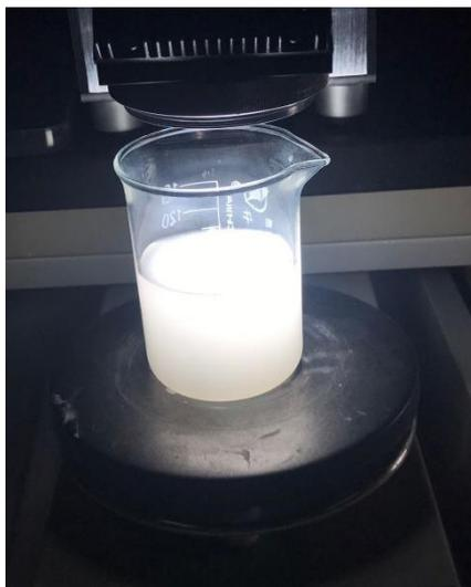
*Figure S1.* A photo of the experiment of in-situ photodeposition in air. The color of suspension remained white.
