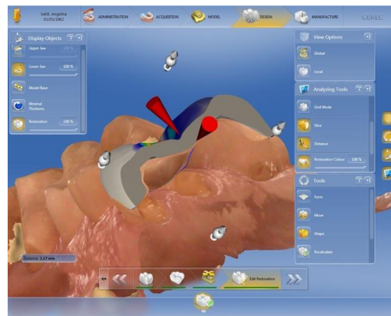
Figure 2. CAD design of tabletop restorations, controlling standardized anatomy and thickness.
