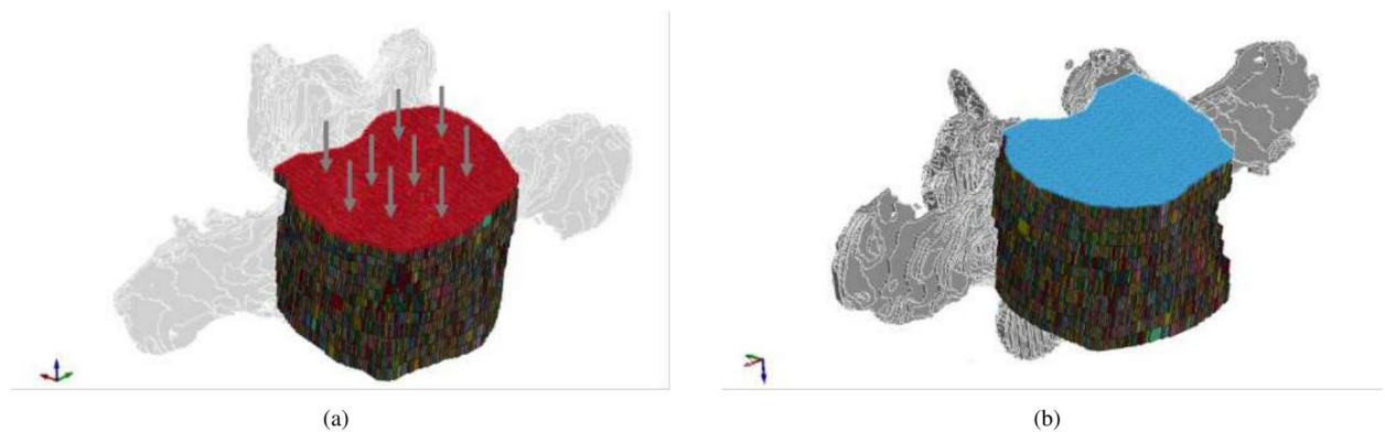
Fig. 5. The distribution of the force applied on the vertebral body. (a) The grey arrows on the red area represent the 1000 N force exerted on the upper surface; (b) the blue area represents the fully constrained lower surface with 6 degrees of freedom.
