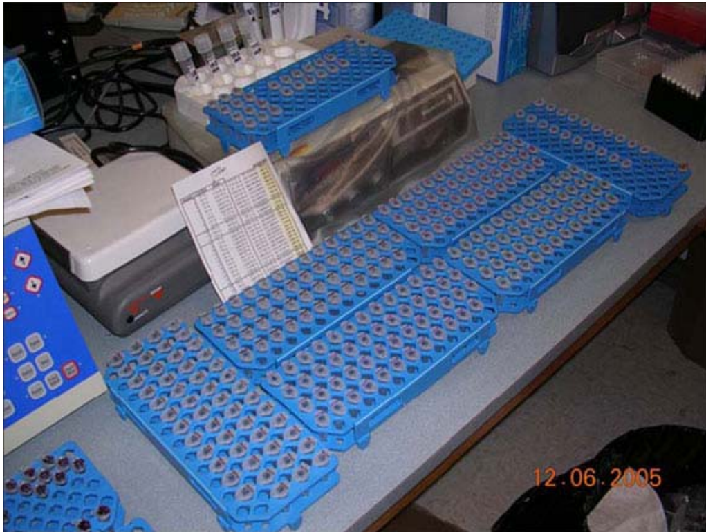
Fig. 43: Typical master mix reaction tube set-up illustrating the often extensive nature of hands-on real-time qPCR. Approximately 260 tubes containing optimally-diluted sample RNAs are not shown here. All tube set-ups were quickly defined by the FF2-6-001 qPCR set-up tool.
