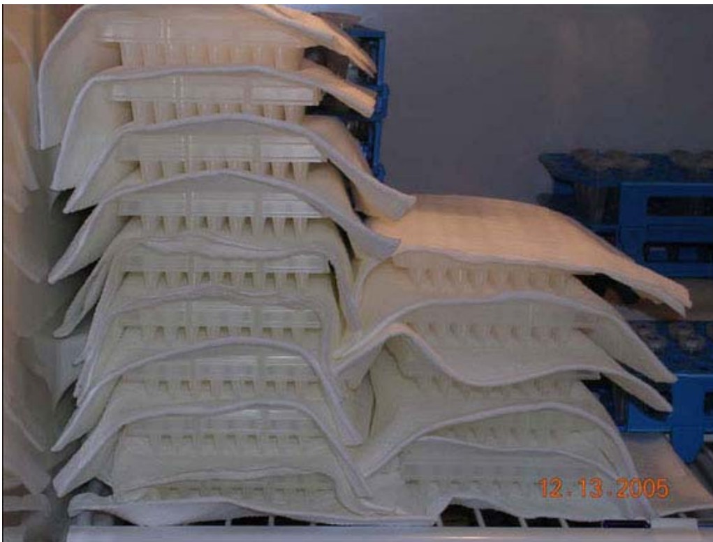
Fig. 44: Typical storage of fluorogenic one-step real-time qPCR plates at 4 °C before being run. In the example shown here, it took one person 42 hours to run all 14 plates back-to-back. Liquid-handling robot technology has been welcomed in many labs on account of the elaborate, time-consuming set-ups that frequently accompany truly interrogative qPCR. Electronic pipettes can be used otherwise to help shorten set-up time.
