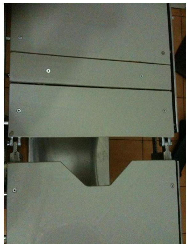
Figure 1 Operation Theatre Table Top. Still Image showing operation theatre table top with gap between the table attachments.
