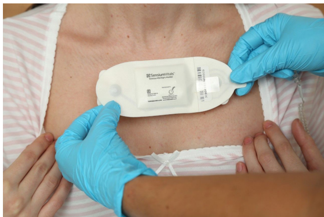
Figure 1 The SensiumVitals monitoring patch. Image reproduced with permission from Sensium, Abingdon, UK.
