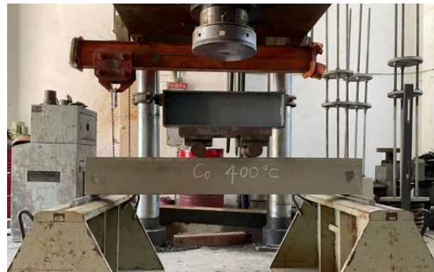
Figure 4. The general flexural test setup for the beam specimens.
