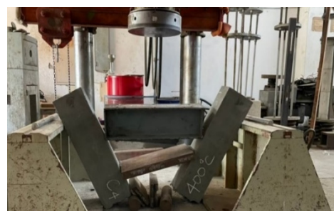
Figure 12. The fracture situation of the experimental group after being subjected to 400 °C.
