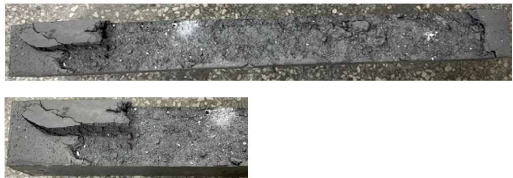
Figure 9. The spalled surface of the UHPC beam specimen after being subjected to 500 °C.
