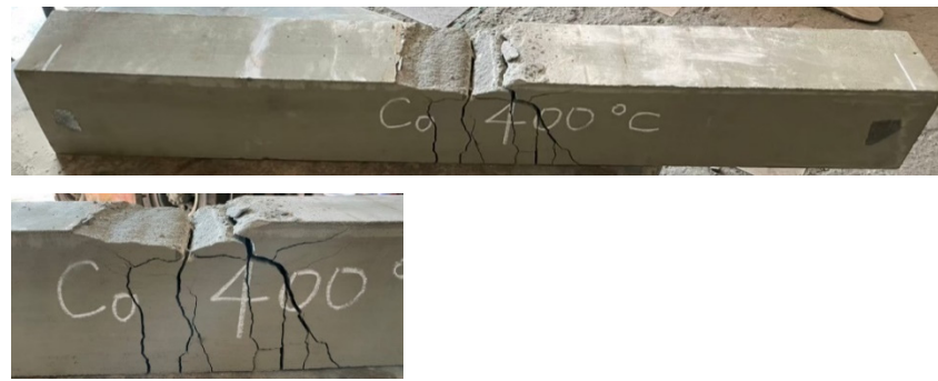
Figure 13. The distribution of the flexural cracks of the control group after being subjected to 400 °C.
