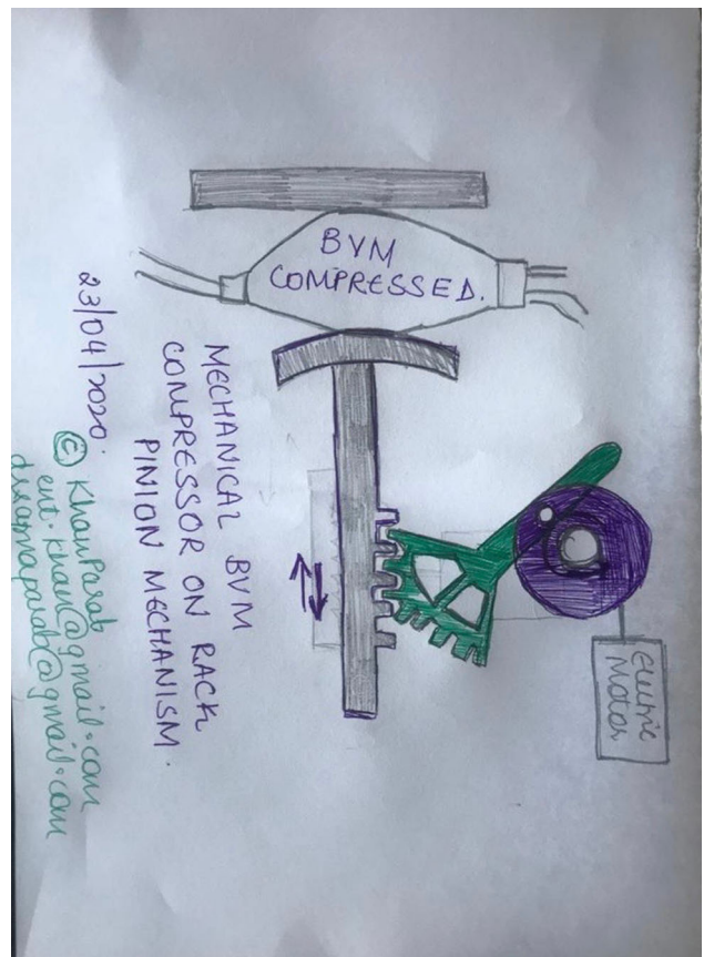
Fig. 3 Alternate model for mechanical Bag Valve Mask compression
