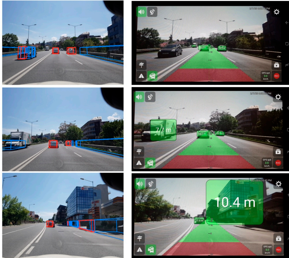
Figure 15. Comparison with a CNN-based detector running on mobile devices. Left column—our approach, right column—UGV Driver Assistant.
