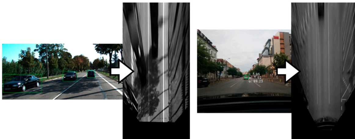
Figure 14. Generating the Inverse Perspective Mapping (IPM) image using the calibration data.
