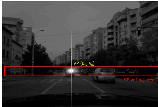
Figure 11. Finding the vanishing point (VP). The road edges will vote in the area around the already estimated horizon row, and the position with the maximum votes will be selected as the vanishing point.
