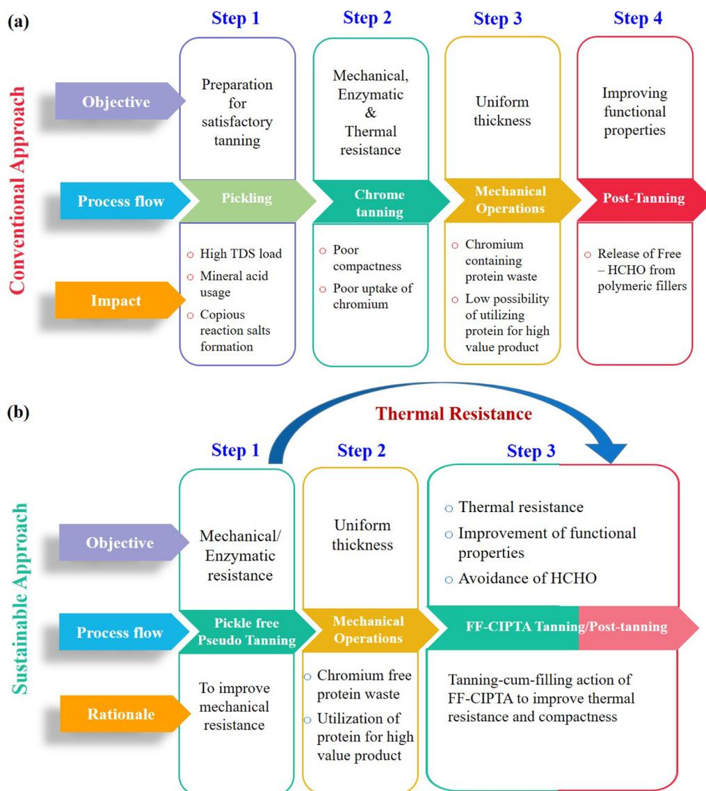
**Figure 1.** Process flow diagram of (a) conventional and (b) sustainable approach.
