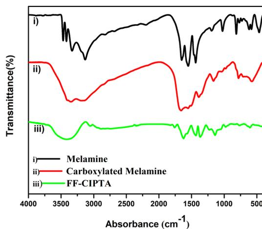
**Figure 3.** FT-IR spectrum of (i) melamine, (ii) CM, (iii) chromium incorporated polymeric tanning agent (FF-CIPTA).
