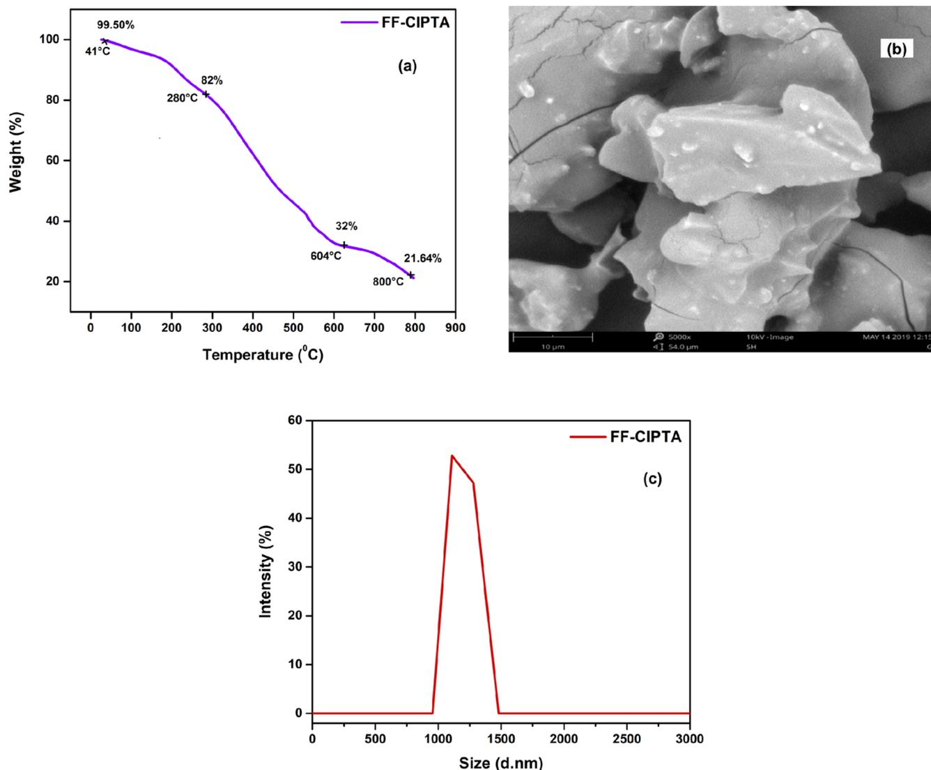
**Figure 4.** (a) Thermogravimetric curve of FF-CIPTA, (b) SEM micrograph of FF-CIPTA at a magnification of 5000 $\times$ , (c) hydrodynamic size of FF-CIPTA.
