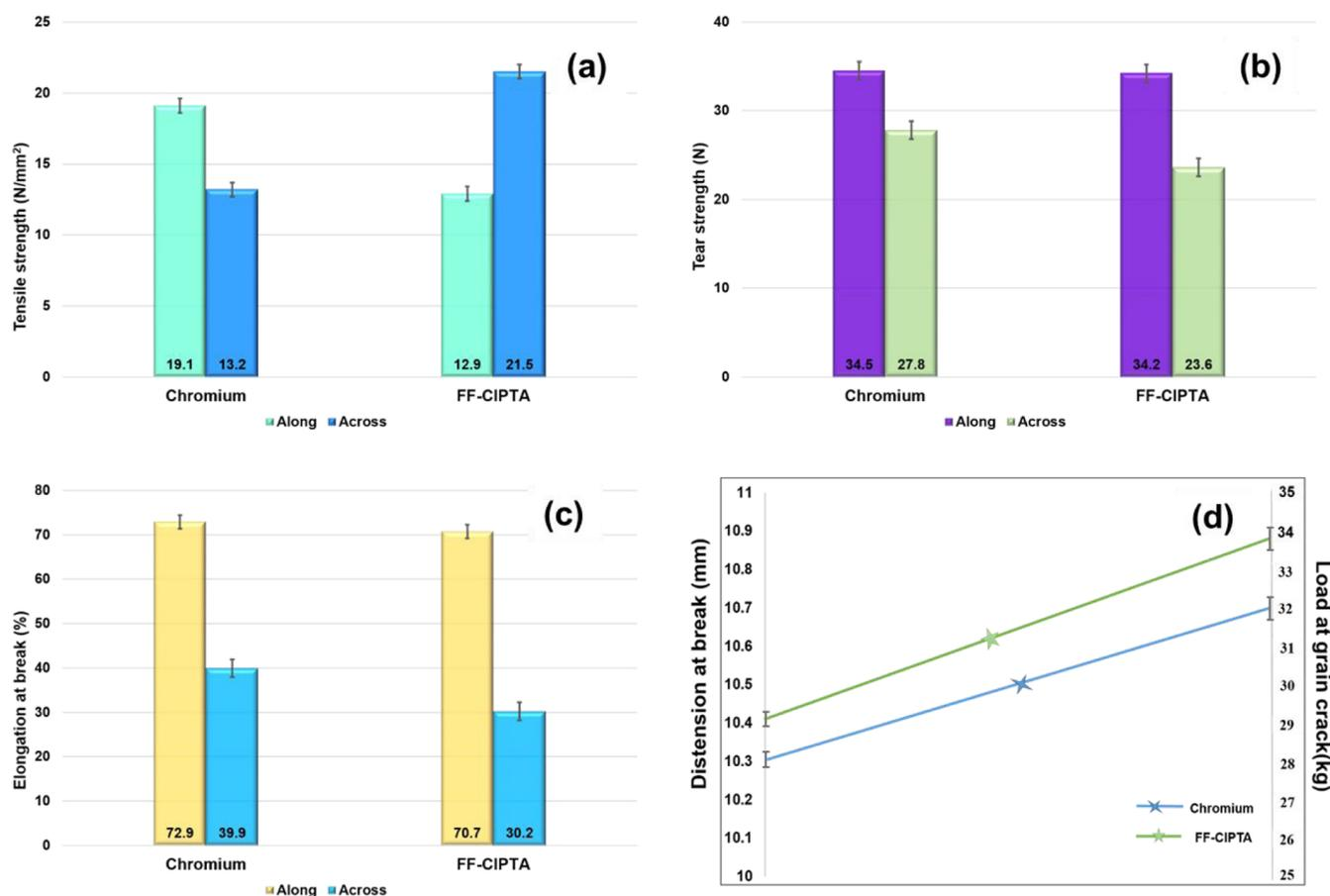
**Figure 8.** Physical strength characteristics of chromium tanned and chromium tanned polymeric crust leathers, (a) tensile strength, (b) tear strength, (c) elongation at break, (d) load at grain crack and distension at break.
