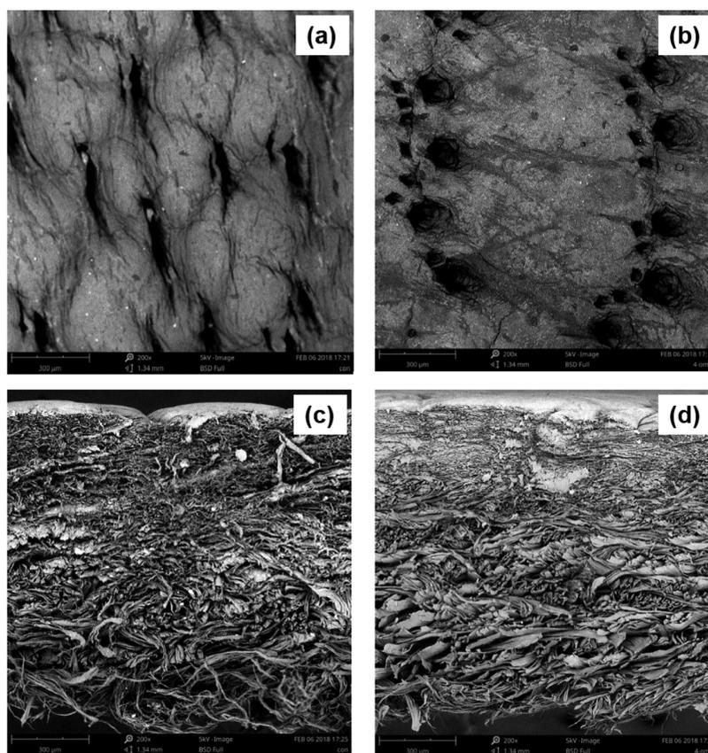
**Figure 6.** SEM micrographs showing the grain surface and cross section of control leather (a,c) and experimental leather (b,d) at a magnification of 200 $\times$ .
