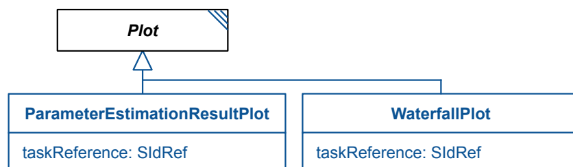
Figure 2.28: The definition of the SED-ML ParameterEstimationResultPlot and WaterfallPlot classes.
