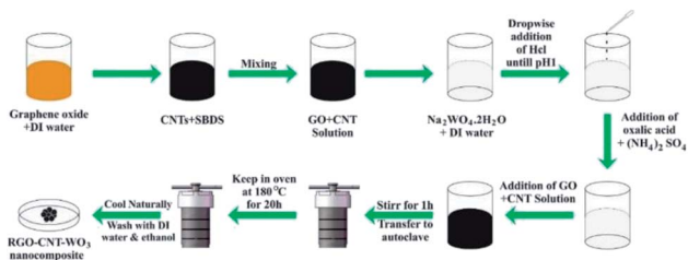
Fig. 2 Schematic diagram of the synthesis of RGO–CNT–WO 3 through hydrothermal method.
