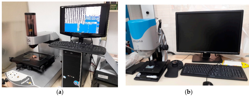
Figure 4. Equipment for surface analysis: (a); digital profile projector TESA-VISIO; (b) optical micro-coordinate measurement machine IF-SL ALICONA.
