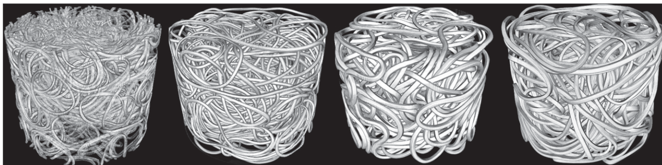
Fig. 1. Packing structure of confined rubber bands. Shown are X-ray tomograms of bands' packing of different lengths. From Left to Right the tomograms correspond to bands of types A, B, C, and E (Table 1).
