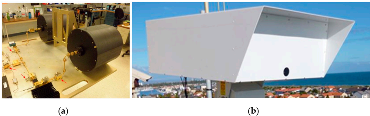
Figure 1. (a) The internal design of the W-band radar showing transmit and receive antennas and RF section; (b) the deployed radar encapsulated by a radome mounted on a pan-tilt positioner and situated at the top of a control tower at the entrance to a busy port.
