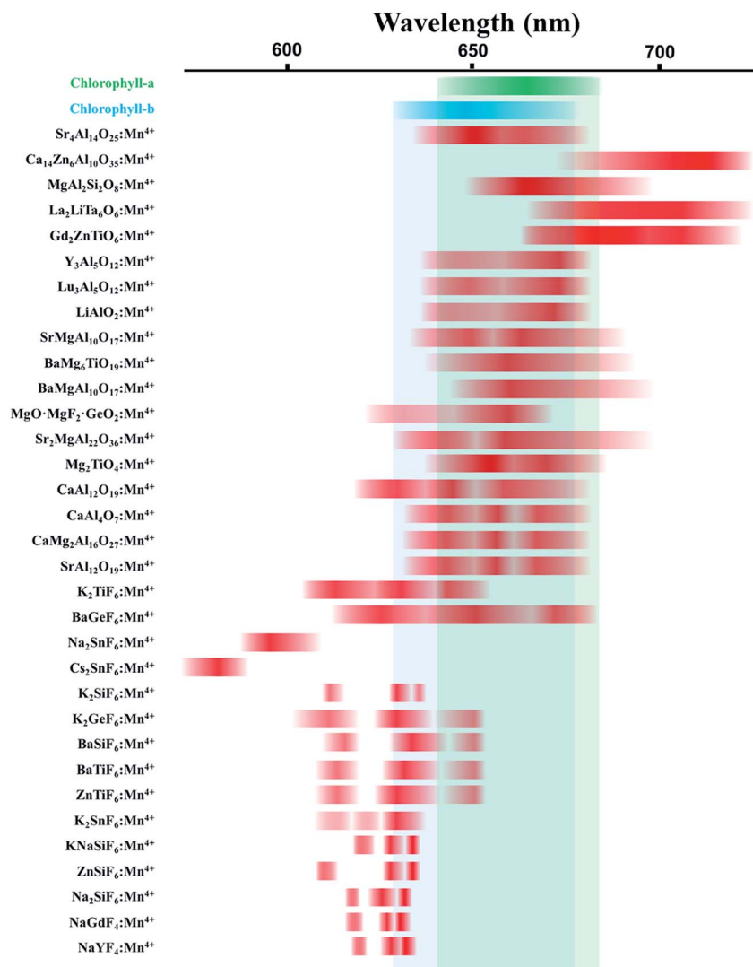
Fig. 1 Spectroscopic range of \text{Mn}^{4+} ions in various crystals. Green and blue color indicate the absorption spectrum region of chlorophyll-a and chlorophyll-b, respectively. Red color indicates the emission spectrum region of various phosphors with \text{Mn}^{4+} ions doped.
