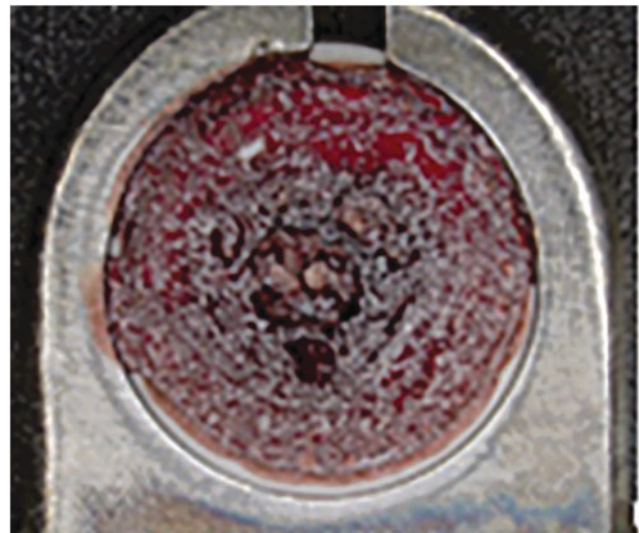
FIG. 2. Jig for attaching RFID tag after contaminants added. Color image is available online.
