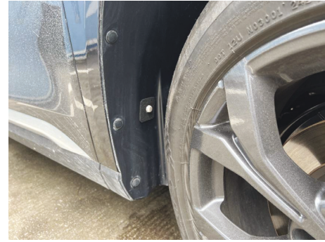
FIGURE 2: The humidity sensor behind a car tire.
