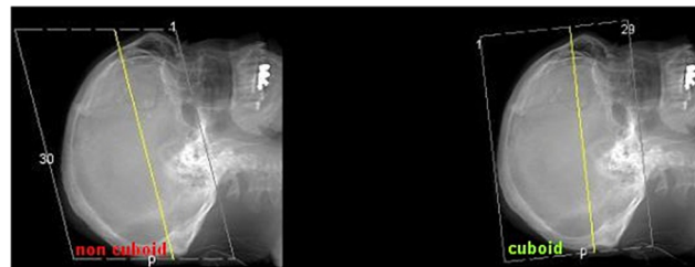
Fig 9. In order to be able to apply Pythagoras' theorem, the line “travelled” by the cursor through the slices must be vertical to the slice orientation. This is only the case if the slices are “piled aligned” in a cuboid dataset ( right ). If the gantry angle is modified during data acquisition, the resulting dataset is a non-cuboid parallelepiped, and the calculation cannot be applied. In that case, a cuboid dataset can be reconstructed at the CT workstation. Whether the regarded slices are applicable for the caliper navigation technique or not can be seen at a glance in the corresponding scout.
