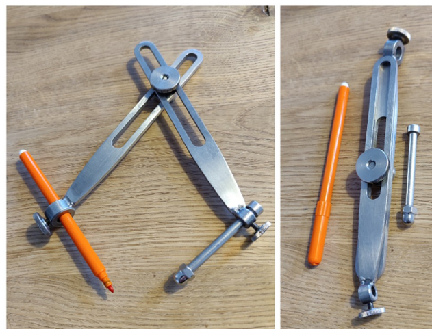
Fig 7. Craniotomy caliper. The demands to a caliper to facilitate the marking part of this method have been addressed in this model designed by the first author: The contact point of the center leg is smooth and can be inserted to the porus and placed on nasion. The length of legs of the caliper can be adjusted and together with the fix angle chosen for the mounting rings, this length adjustment allows to keep the angle of the center leg and the marker nearly vertical to the skin at all different convexity locations, which reduces the error. The mounting rings allow to insert different diameters of markers. The tool can be folded up and fits in a pocket.
