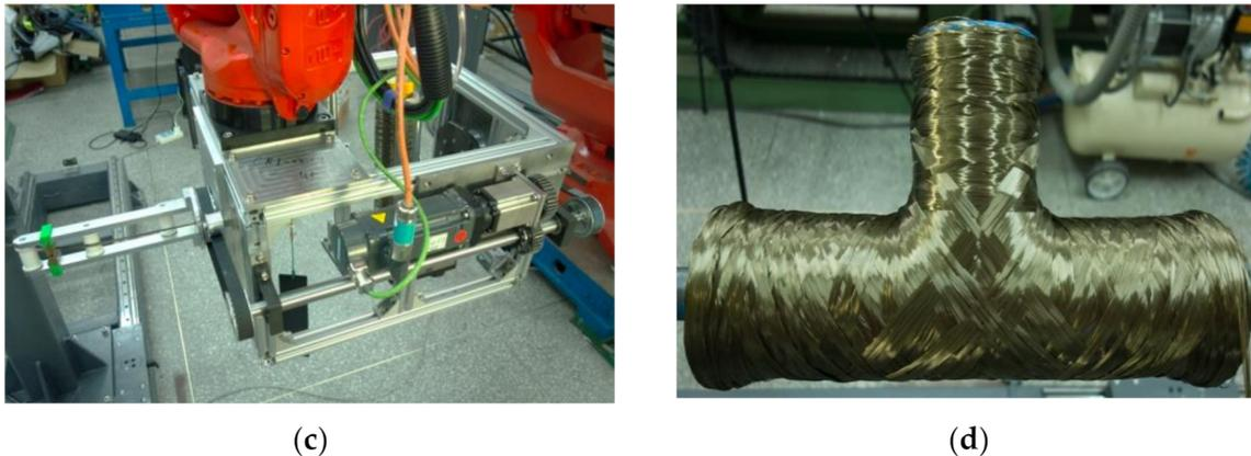
**Figure 14.** Six-axis robot winding system: (a) Winding head structure; (b) Six-axis robot; (c) Winding head; (d) Tee pipe after winding.
