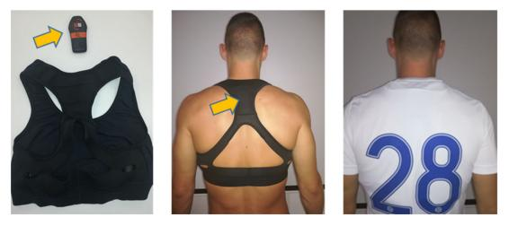
Figure 1. Global positioning device (GPS) used for the measurement of running performances in soccer.
